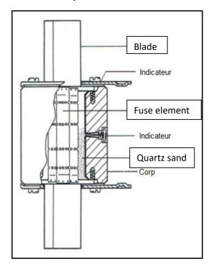
The NH00C range of fuses with gG size 00 fusing characteristics is available with current ratings from 50A to 1600A.
